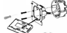
3. Connect the LCD board into the wallplate.
