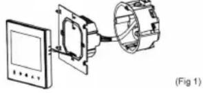
2. Fix the wall plate into the wall box by a screwdriver
