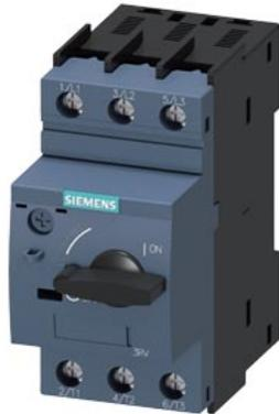
Circuit breaker 20 A A-release 13...20 A, N-release 260 A, for motor protection, class 10, screw connection, standard switching capacity
