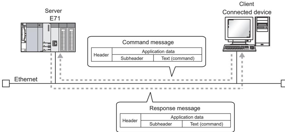
The frames that can be used with an E71 are as follows.
