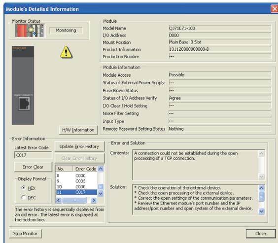
3. The "Module's Detailed Information" window is displayed. Clicking the **Update Error History** button displays the error details and corrective action.
