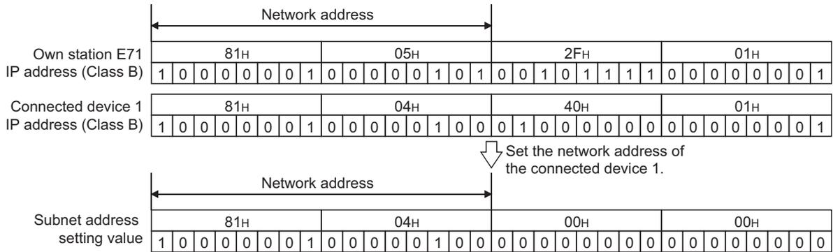
**Ex.** When the classes differ between the E71 on the own station and the connected device
