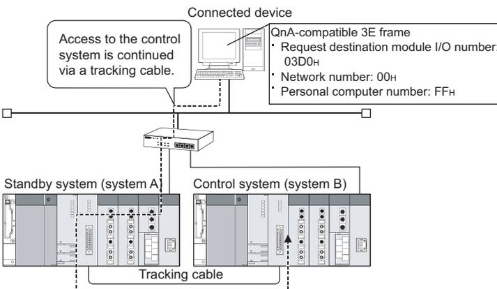
**2.** When the system is switched, the connected device automatically continues access to the control system through the tracking cable. However, if the communication line with the connection destination is faulty or the standby system is powered off, for example, the destination must be changed on the connected device.
