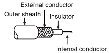
● The following shows how to attach the BNC connector and the coaxial cable.
