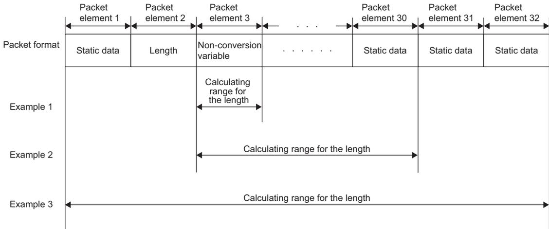
Example 1) Calculating range when its start is 3 and end is 3
