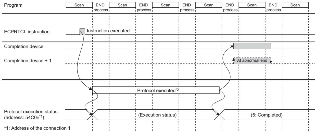
\*2: Protocols are consecutively executed by the number of protocols specified in n2 of the setting data in the order specified with the control data (up to eight protocols) with one ECPRTCL instruction.
