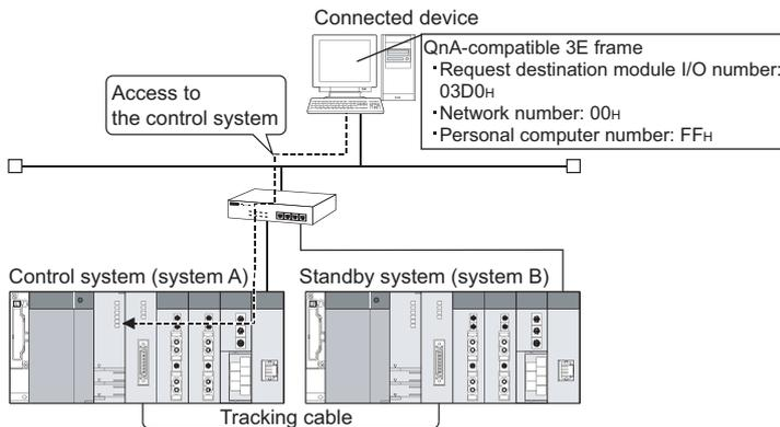
**1.** Connect the connected device to the E71 mounted with the control system CPU module to access the control system CPU module.
