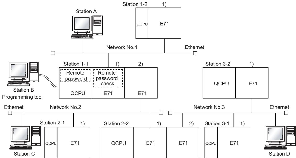
\*1 The station A is the only connected device that can perform an unlock/lock process for 1) of the station 1-1.
