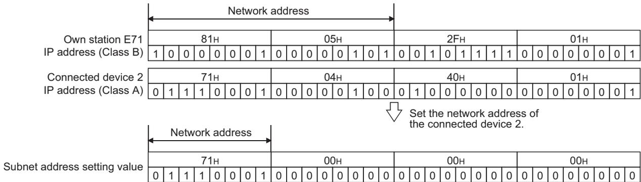
**Ex.** When the network address of the E71 on the own station is the same as that of the connected device
