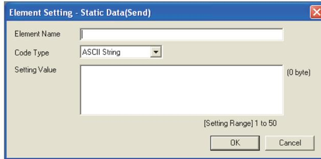
This element is used when a specific code or character string such as a command exists in a packet.
