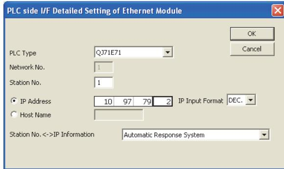
**4.** Select "Ethernet Module" under "PLC side I/F" and double-click the item. The window shown to left appears. Set the station number and the IP address according to the network parameters.
