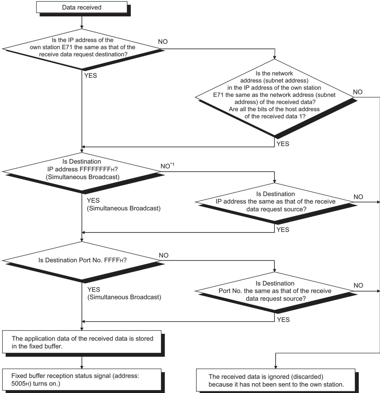
\*1 When all the bits of the area expressing the host address of the IP address of the receive data request destination are 1, proceed to "YES".
