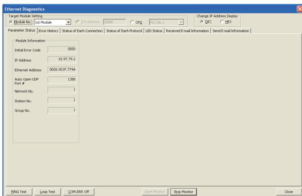
1. Click the **PING Test** button in the "Ethernet Diagnostics" window.
