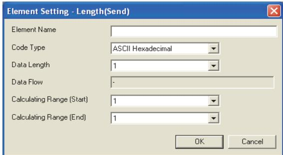
This element is used when an element indicating the data length is included in a packet.
