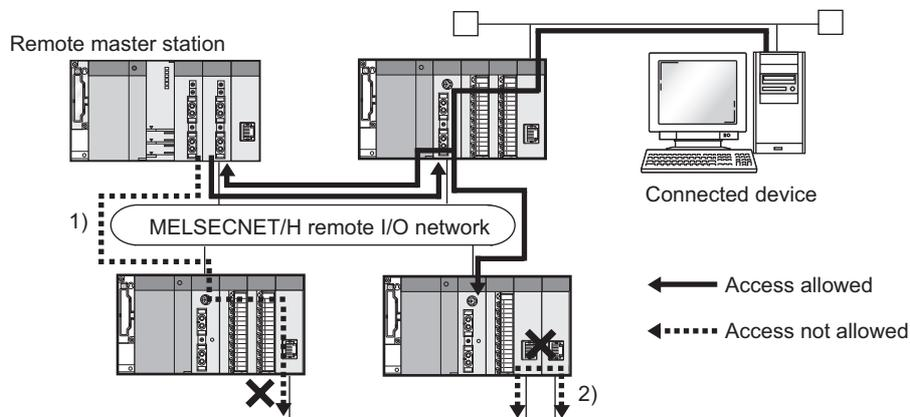
The following methods cannot be used to access other stations through MELSECNET/H remote I/O stations.
