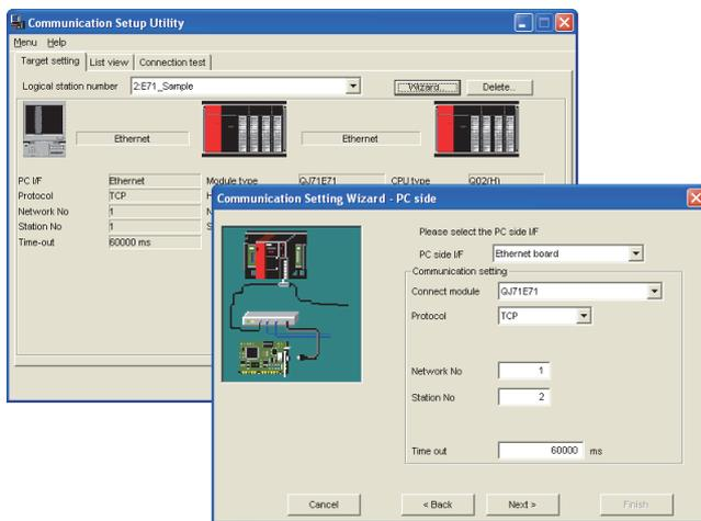
1. Follow the wizard to configure communication settings from the personal computer to the programmable controller. (For some controllers, settings are configured only using the program, without using any wizard.) In the wizard, configure necessary settings such as a logical station number, connection module type, and connection destination programmable controller.
