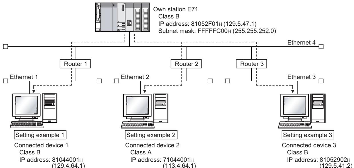
**Ex.** When the network addresses differ between the E71 on the own station and the connected device
