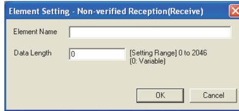
This element is used when receive data include unnecessary data.
