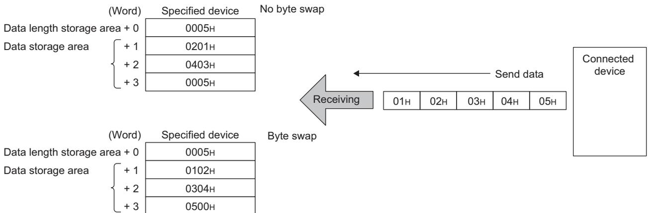
When the setting for "Unit of Stored Data" is "Lower Bytes Only"
