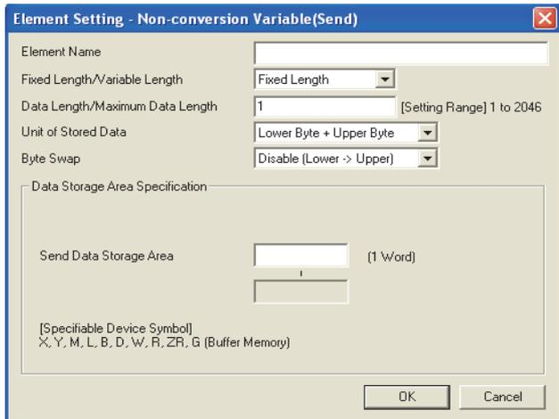
This element is used to send data in the device memory of a CPU module or buffer memory as a part of a send packet, or to store a part of a receive packet to the device memory of a CPU module device or buffer memory. The following table lists the items.
