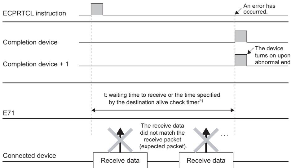
\*1 When the receive packet (expected packet) is not matched to the data by the waiting time to receive or when the existence of a connected device cannot be checked within the time specified by the destination alive check timer (the time calculated based on the destination existence confirmation starting interval timer value, destination existence confirmation interval timer value, and Destination existence confirmation resending time), the instruction ends abnormally.
