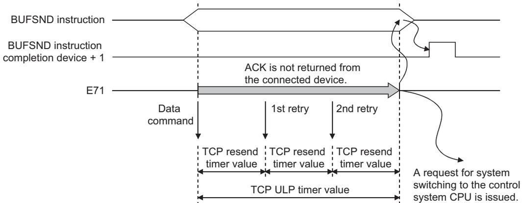
\*2 Set whether to issue the system switching request in the redundant settings of the programming tool. (☞ Page 223, Section 14.7.3)
