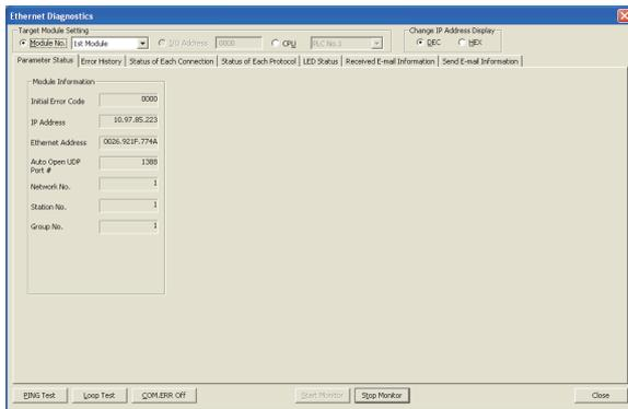
1. Click the **Loop Test** button in the "Ethernet Diagnostics" window.
