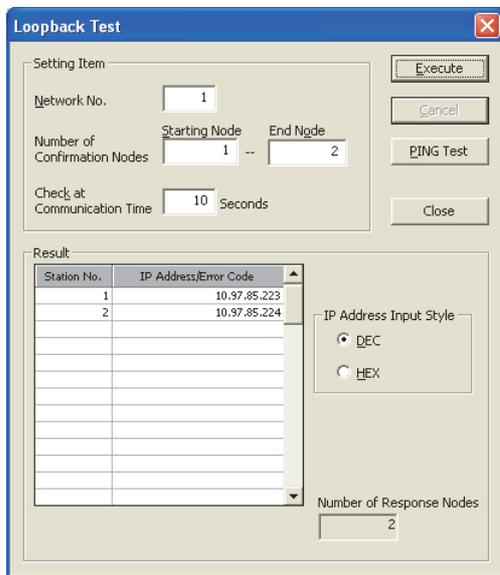
2. Configure the settings and click the **Execute** button to display the test results.
