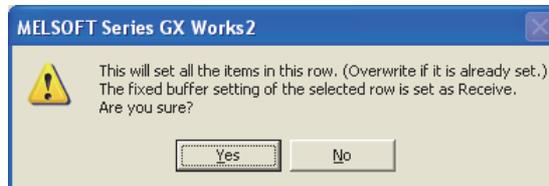
When "Yes" is selected, the applicable connection becomes a receive connection, and the next connection is automatically set as a send connection. (When "Enable" has already been set in "Pairing Open", the setting is overwritten.)
