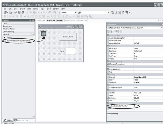
2. Paste the ACT control icon onto the form. Then set the logical station number set in Step 1 to the control as its property.
