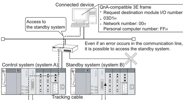
**3.** To access the standby system CPU module, the connected device connects to the E71 mounted with the control system CPU module through the tracking cable. This enables access even if the communication line between the connected device and standby system becomes faulty.
