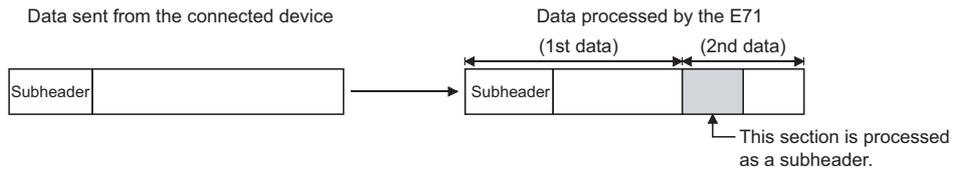
In the figure above, the E71 returns a response containing a code obtained by changing the most significant bit of the code processed as a subheader to 1. For example, if the subheader of a command is 65<sub>H</sub>, the subheader of the response is E5<sub>H</sub>.
