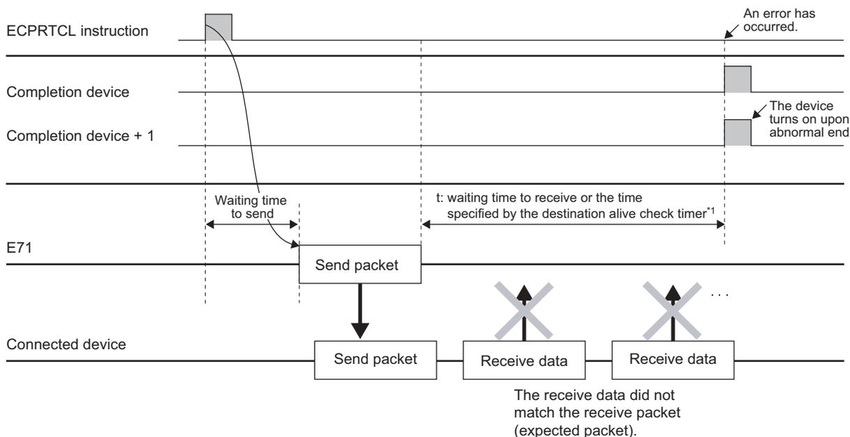
\*1 When the receive packet (expected packet) is not matched to the data by the waiting time to receive or when the existence of a connected device cannot be checked within the time specified by the destination alive check timer<sup>\*1</sup> (the time calculated based on the destination existence confirmation starting interval timer value, destination existence confirmation interval timer value, and Destination existence confirmation resending time), the instruction ends abnormally.
