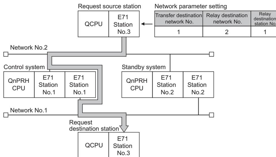
If system switching occurs, change the routing parameter settings using the RTWRITE instruction so that the request source station or relay station accesses the destination through the station of the new control system after system switching.
