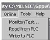
[Monitor/Test] : Activates the Select monitor/test module window.
