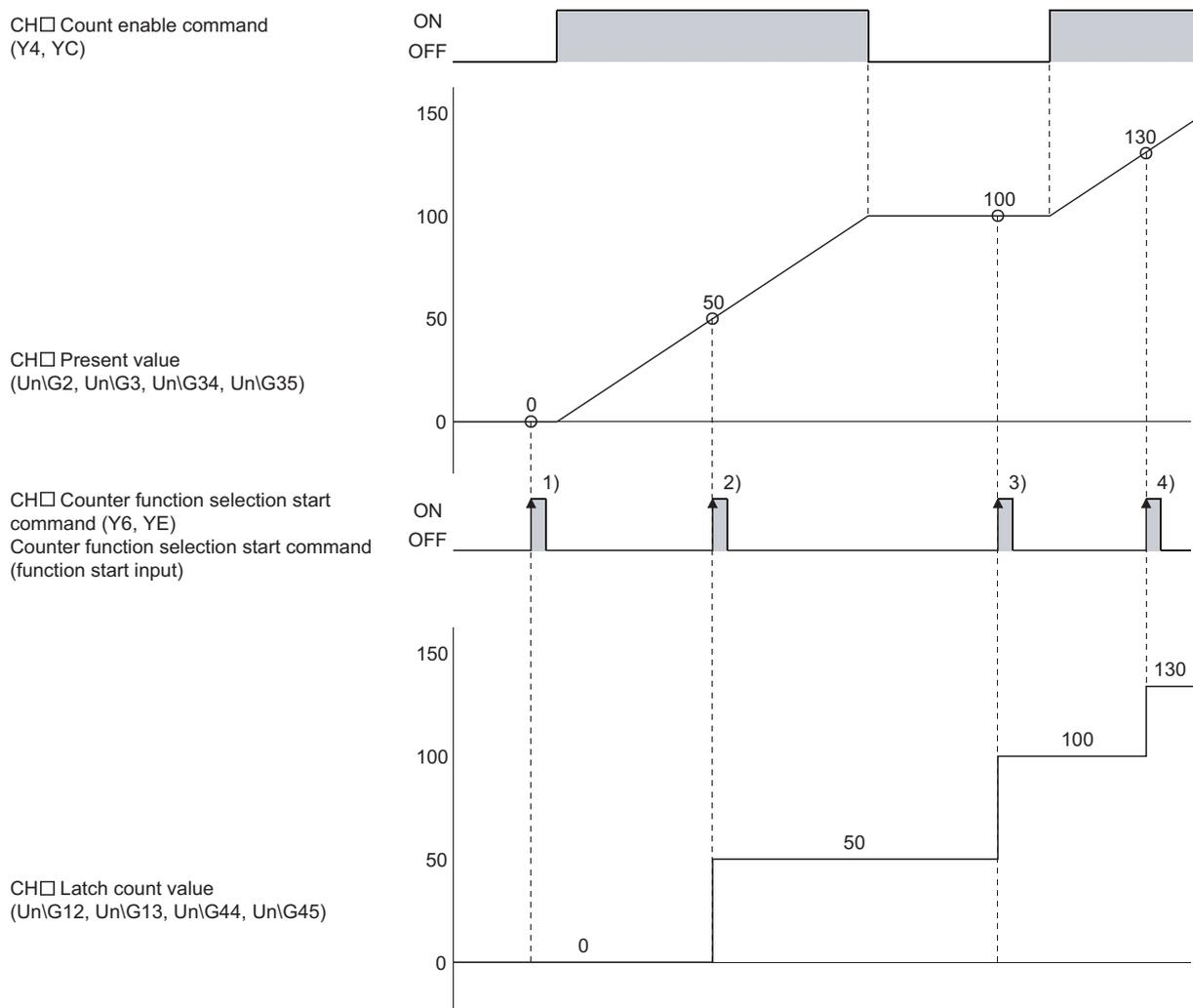
At the rise of CH□ Counter function selection start command (Y6, YE) or the counter function selection start command (function start input) of 1) to 4), the present value of the counter is stored in CH□ Latch count value (Un\G12, Un\G13, Un\G44, Un\G45). The latch counter function can be performed regardless of whether CH□ Count enable command (Y4, YC) is on or off.
