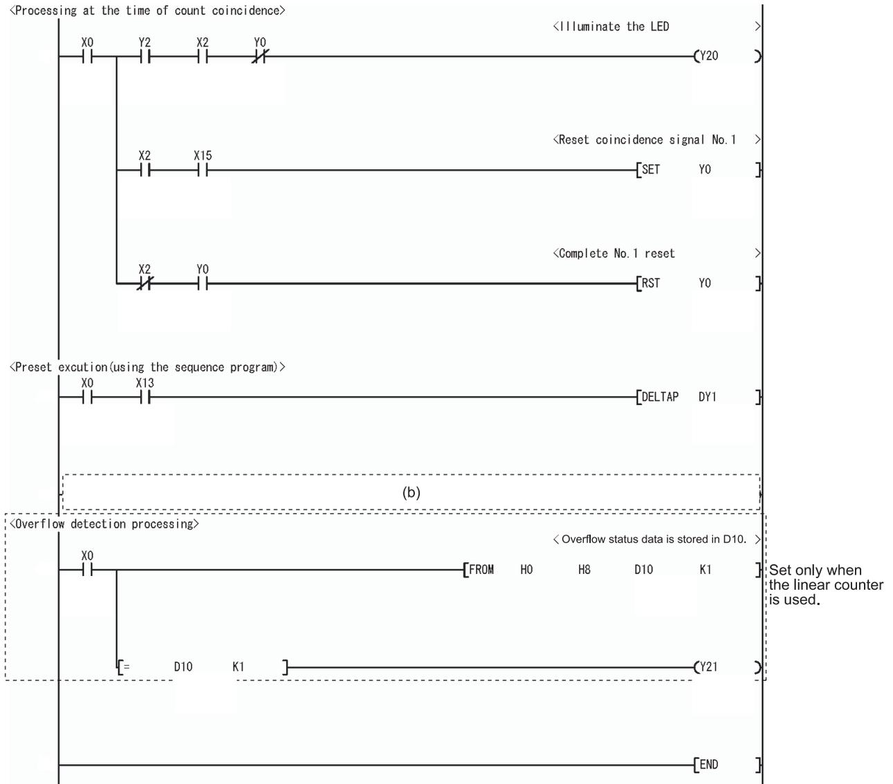
(a) When using the sampling counter function and the periodic pulse counter function, use the following programs.
