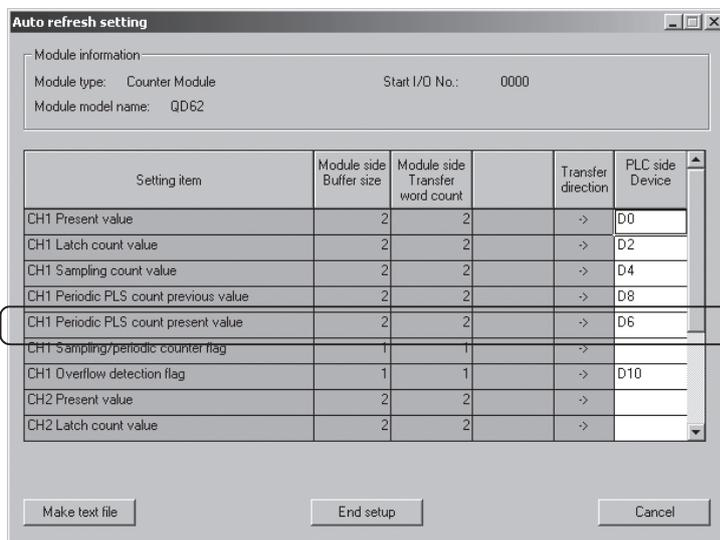
The number of settings in this one line is counted as one setting. The number of settings is not counted by columns. Add up all the setting items in this setting window, then add them to the total for the other intelligent function modules to get a grand total.
