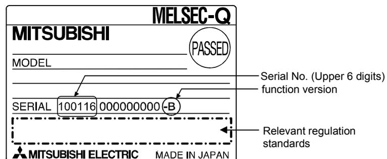
(b) Checking on the front of the module
