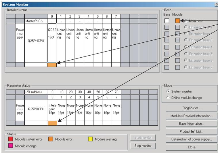
While an overflow error occurs, an orange icon indicating a module error is displayed.
