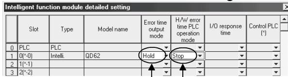
Setting for a CPU stop error      Setting for the QD62 (E/D) error detection
