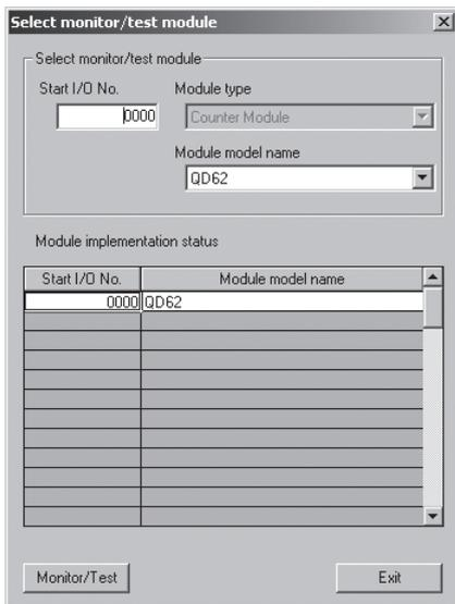
Monitor/test Select a module to be monitored/tested.
