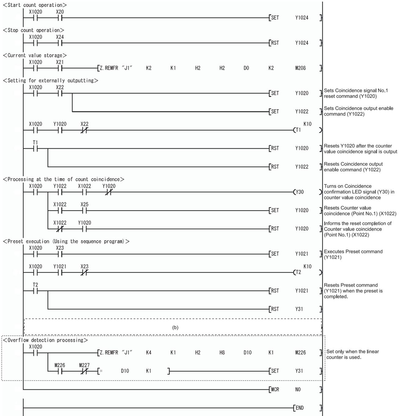
(a) When using the sampling counter function and the periodic pulse counter function, use the following programs.
