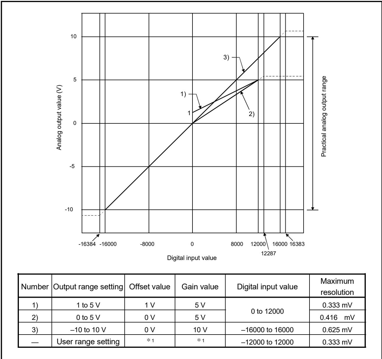
Figure 3.2 Voltage output characteristic in high resolution mode
