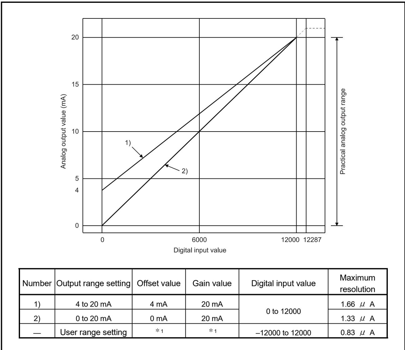
Figure 3.4 Current output characteristic in high resolution mode
