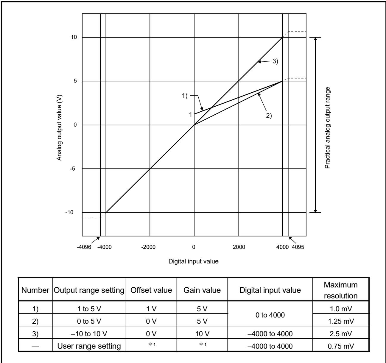
Figure 3.1 Voltage output characteristic in normal resolution mode
