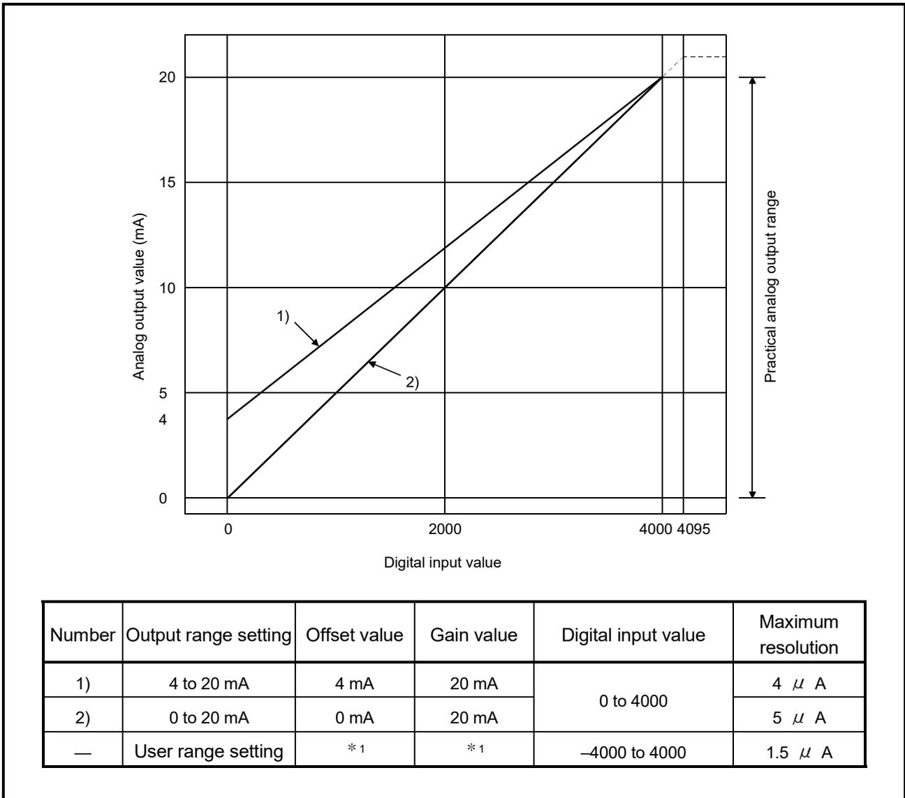
Figure 3.3 Current output characteristic in normal resolution mode
