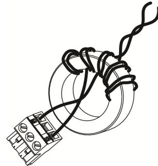
Wire the 24 VAC supply power wires from the transformer to the HOT and COM terminals on the terminal plug as shown in the following figure. The middle terminal on the supply power terminal block is not used. See Table 4 for more information about the Supply Terminal Block.
