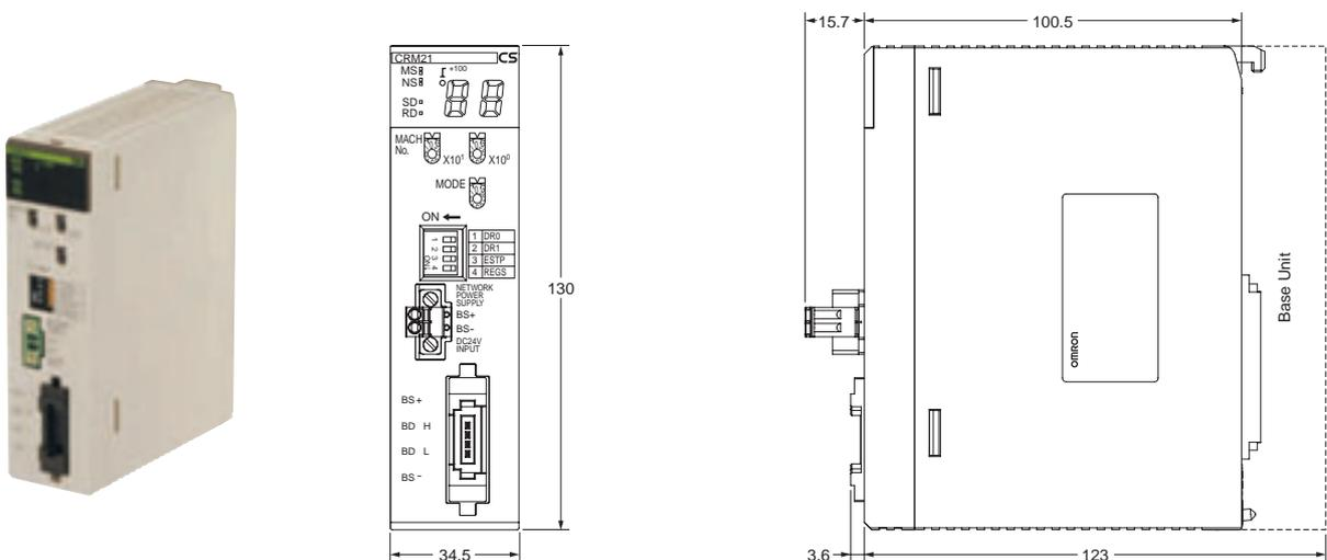
Dimensions When the Cable is Attached
