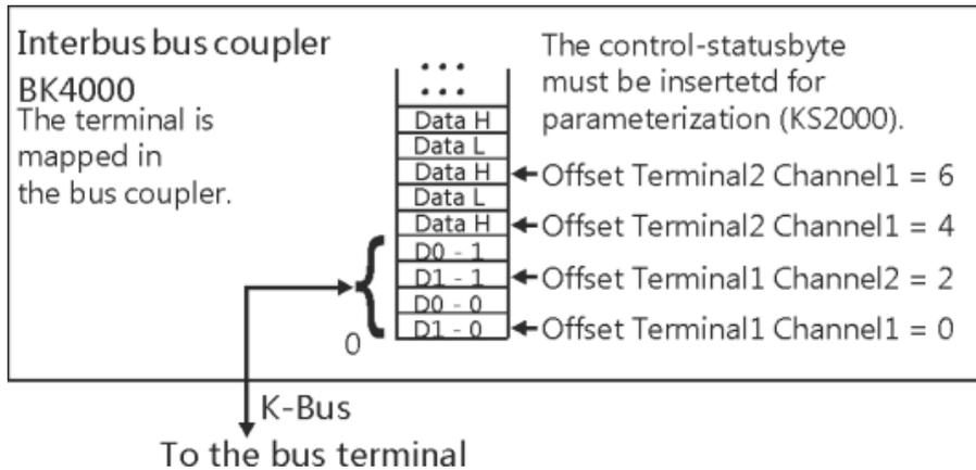
Fig. 16: Mapping in the Interbus coupler – example for KL4002
