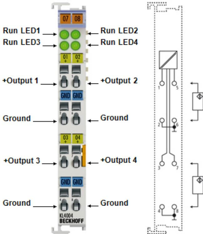
Fig. 12: KL4004 - connection and LEDs
