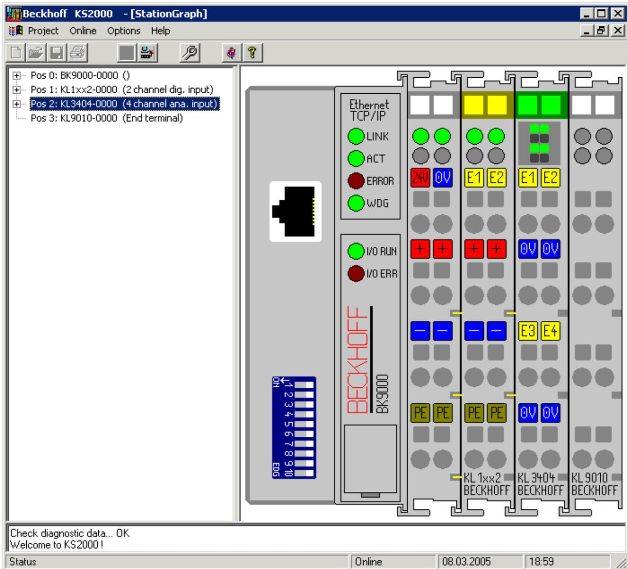
Fig. 18: Display of the fieldbus station in KS2000
