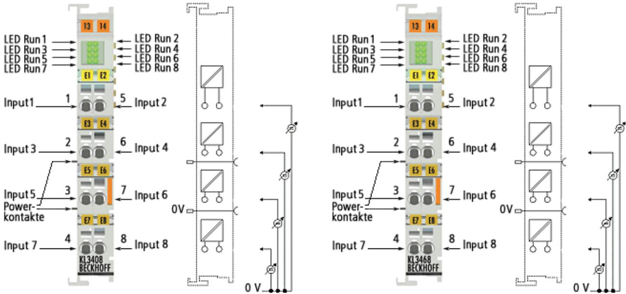
Fig. 16: KL3408 and KL3468 - Contact assignment
