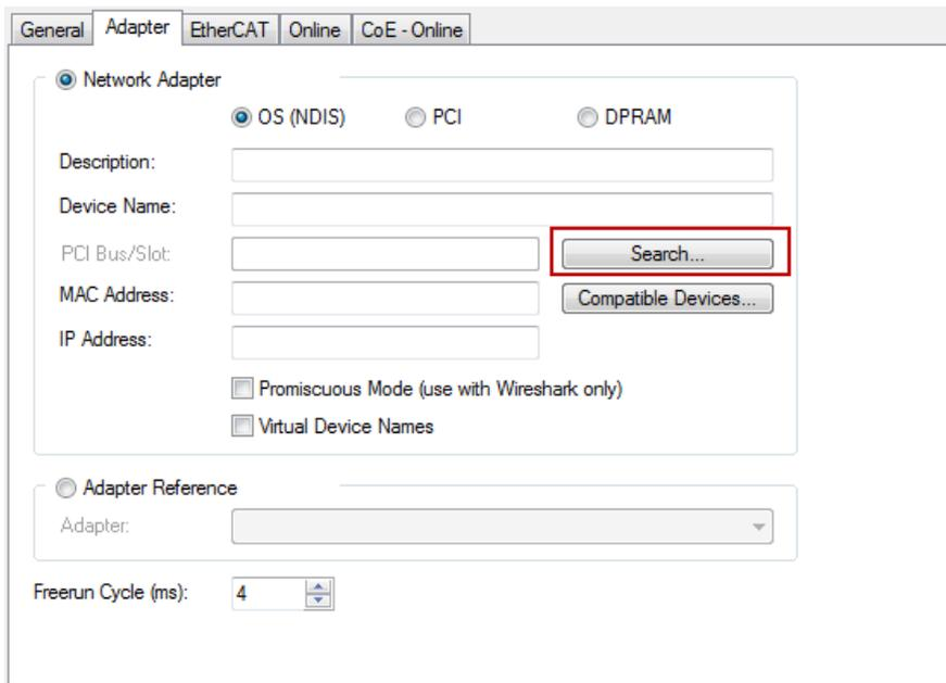
Fig. 24: Search of the existing HW configuration for the EtherCAT configuration of the example
