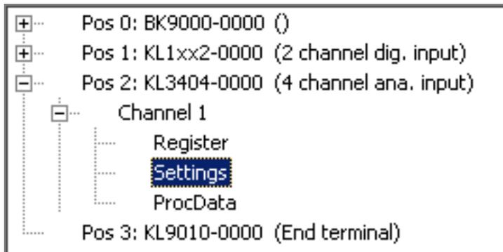
Fig. 19: KS2000 tree branch for channel 1 of the KL3404
