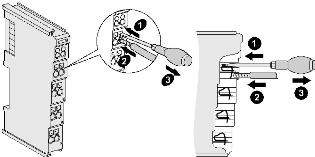
Fig. 14: Connecting a cable on a terminal point
