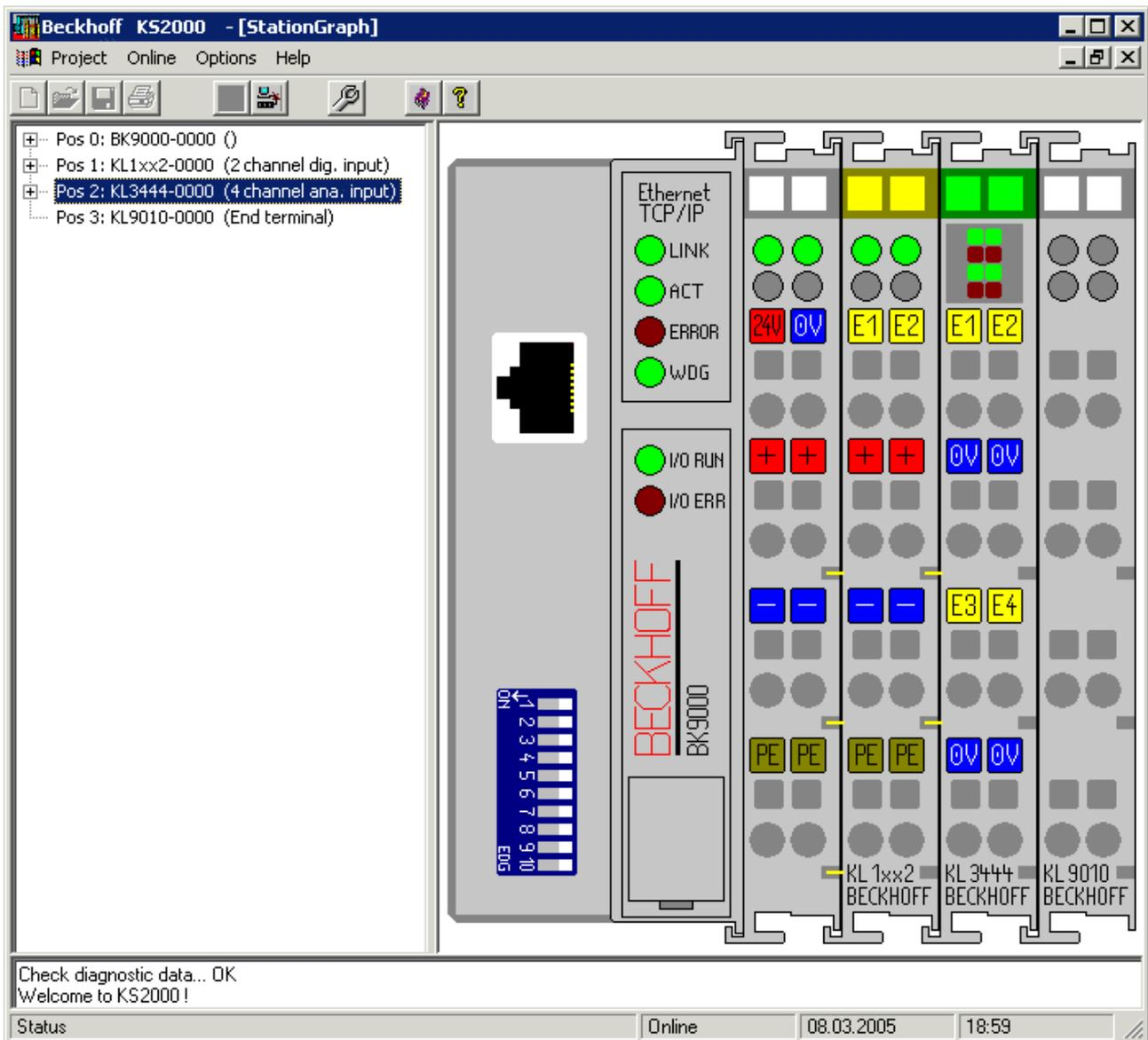
Fig. 22: Display of the fieldbus station in KS2000
