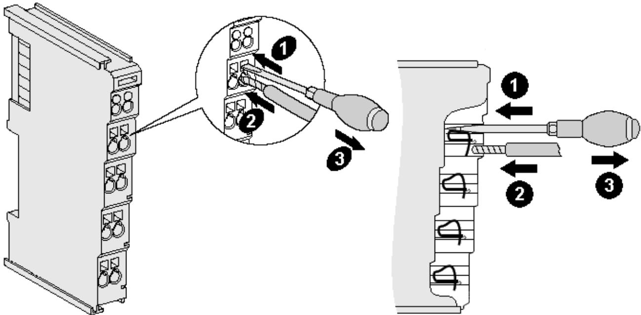
Fig. 17: Connecting a cable on a terminal point
