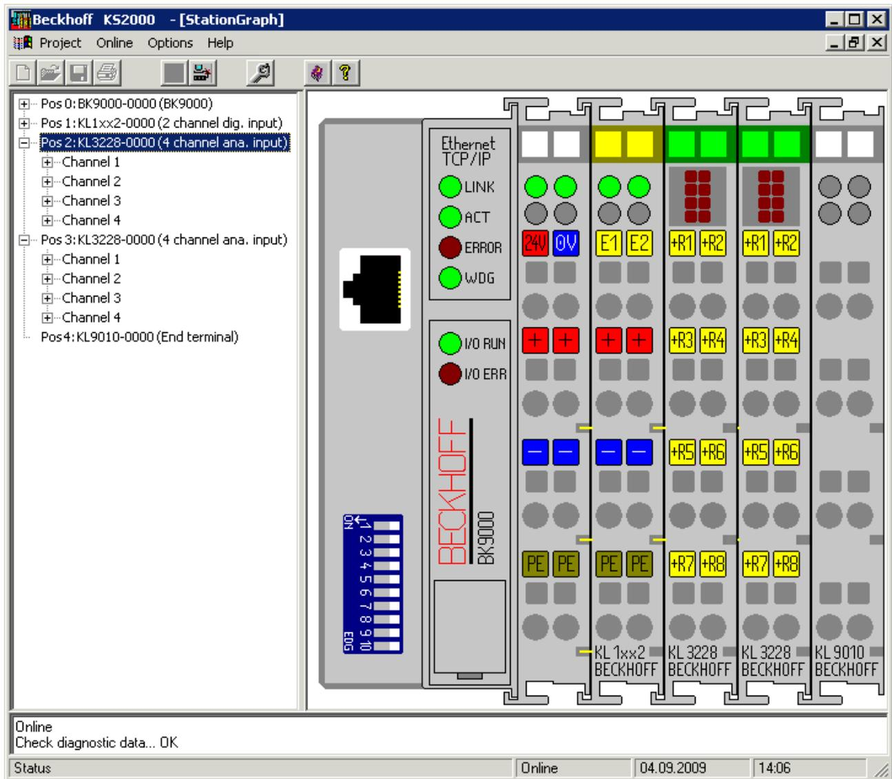
Fig. 17: Display of the fieldbus station in KS2000
