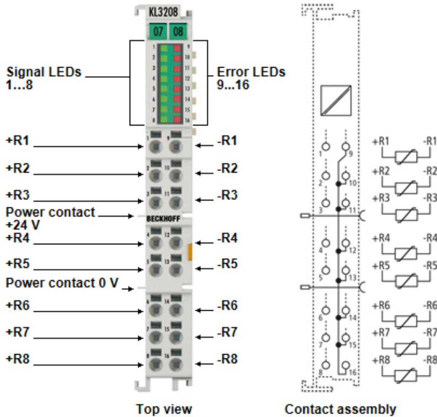
Fig. 12: KL3208-0010 - Contact assignment
