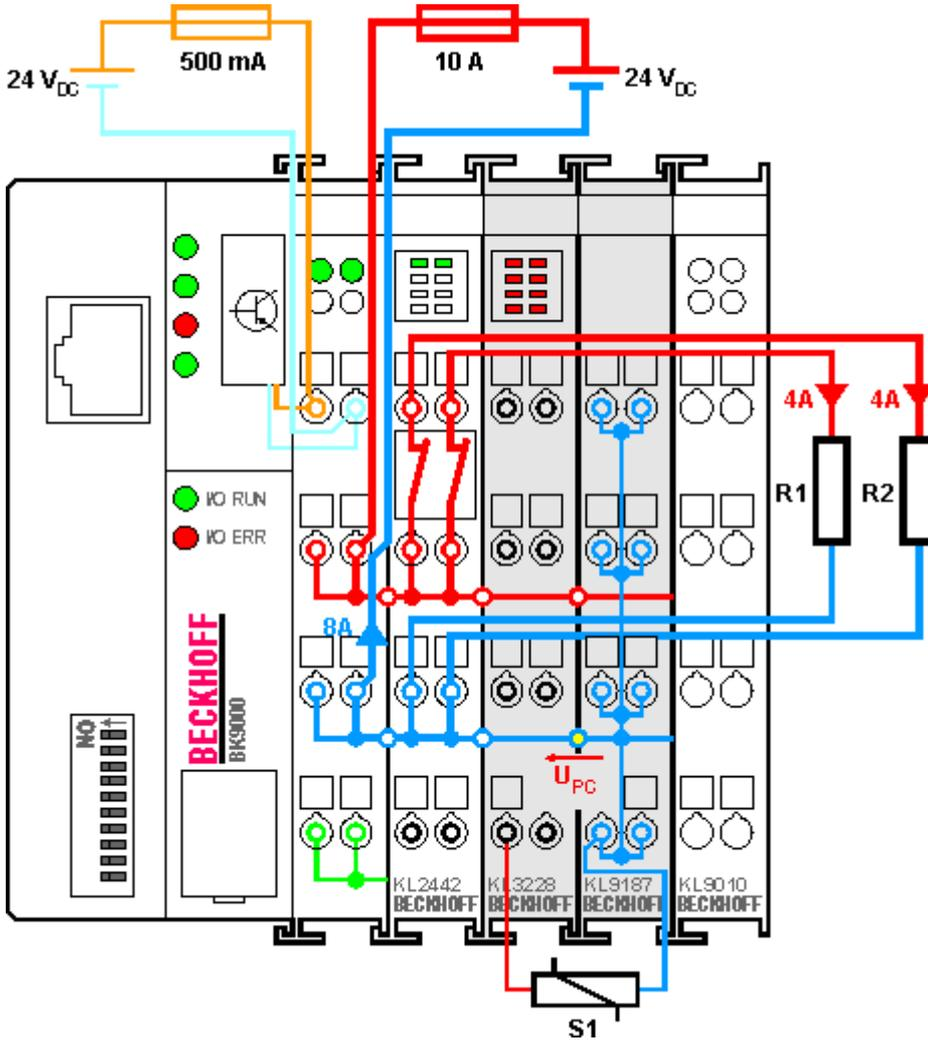
Fig. 15: KL3228/KL9187 - Example for good positioning
