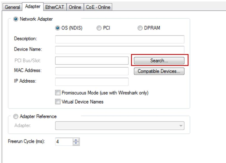
Fig. 23: Search of the existing HW configuration for the EtherCAT configuration of the example
