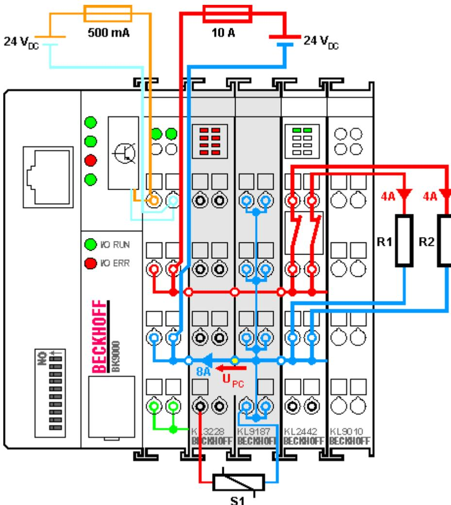
Fig. 14: KL3228/KL9187 - Example for bad positioning
