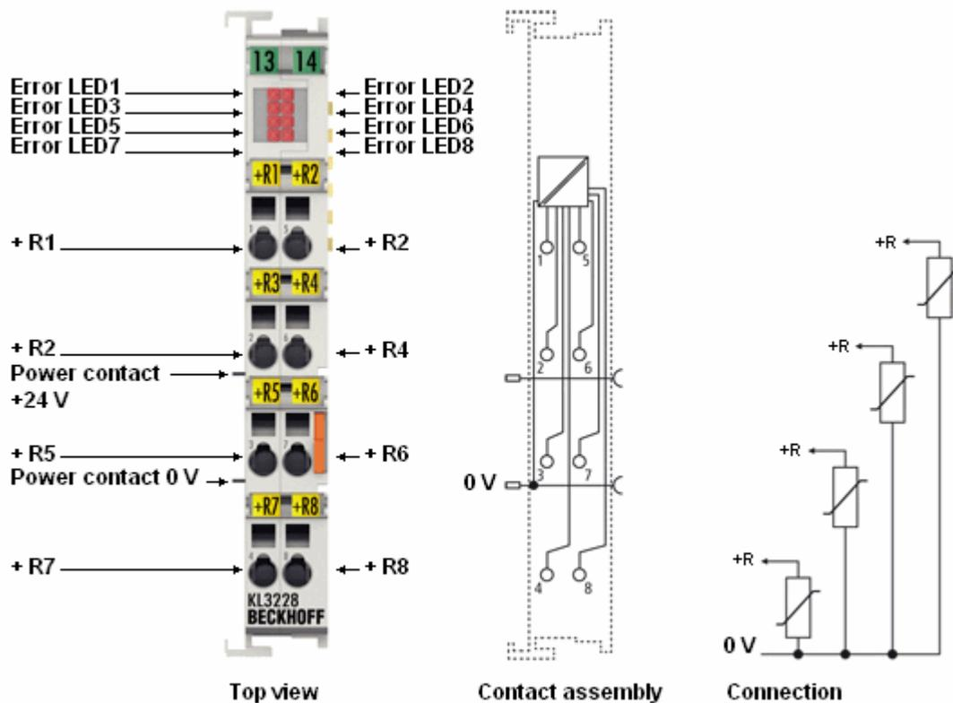
Fig. 13: KL3228-0000 - Contact assignment
