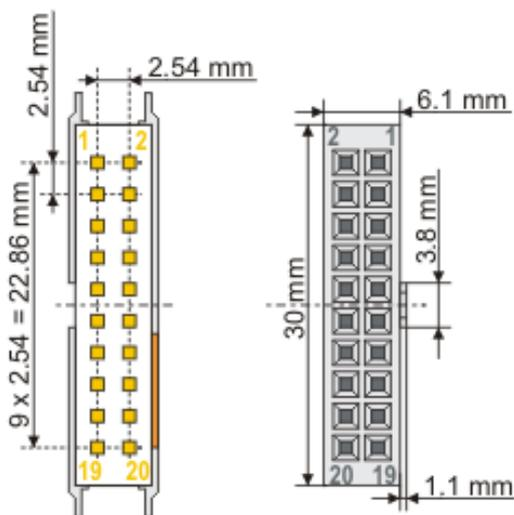
Fig. 10: Dimensions of the 20-pin contact strip in the terminal and the matching spring contact strip
