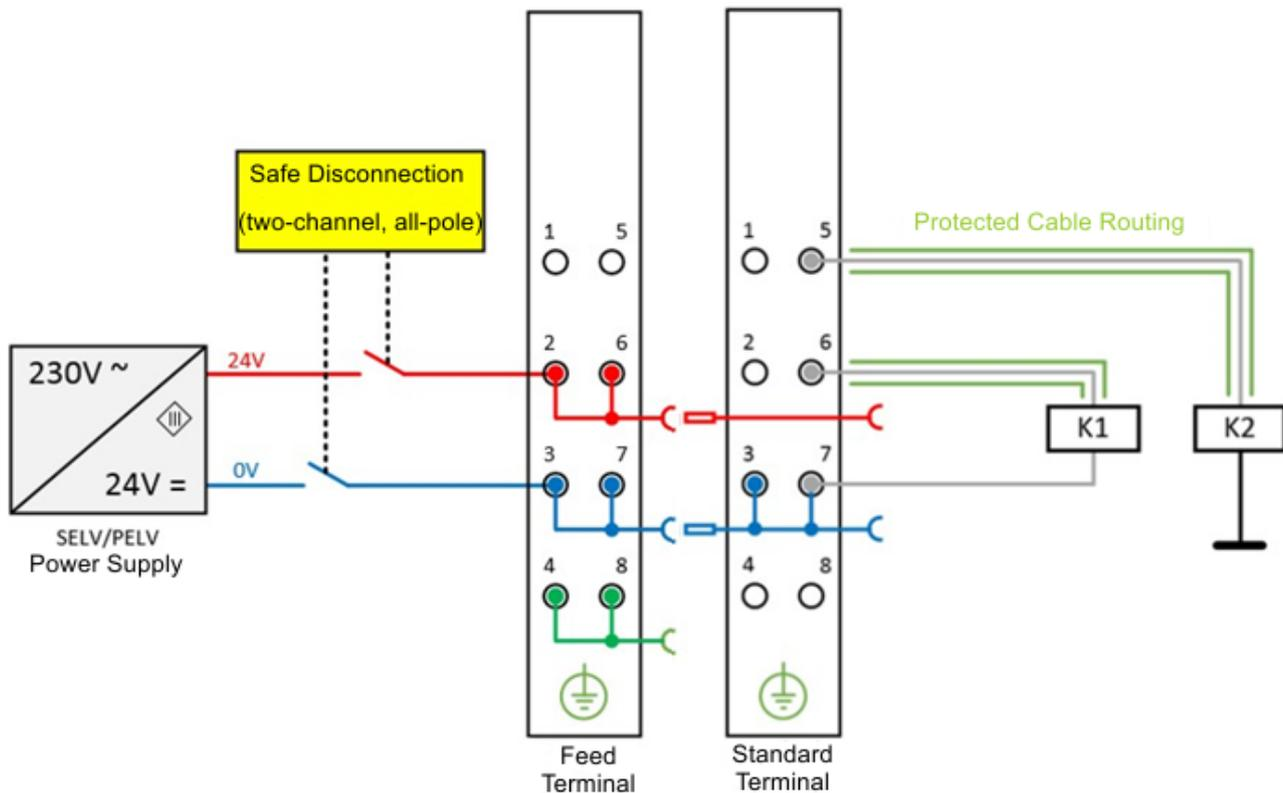
Fig. 3: Short circuit fault exclusion through protected cable laying
