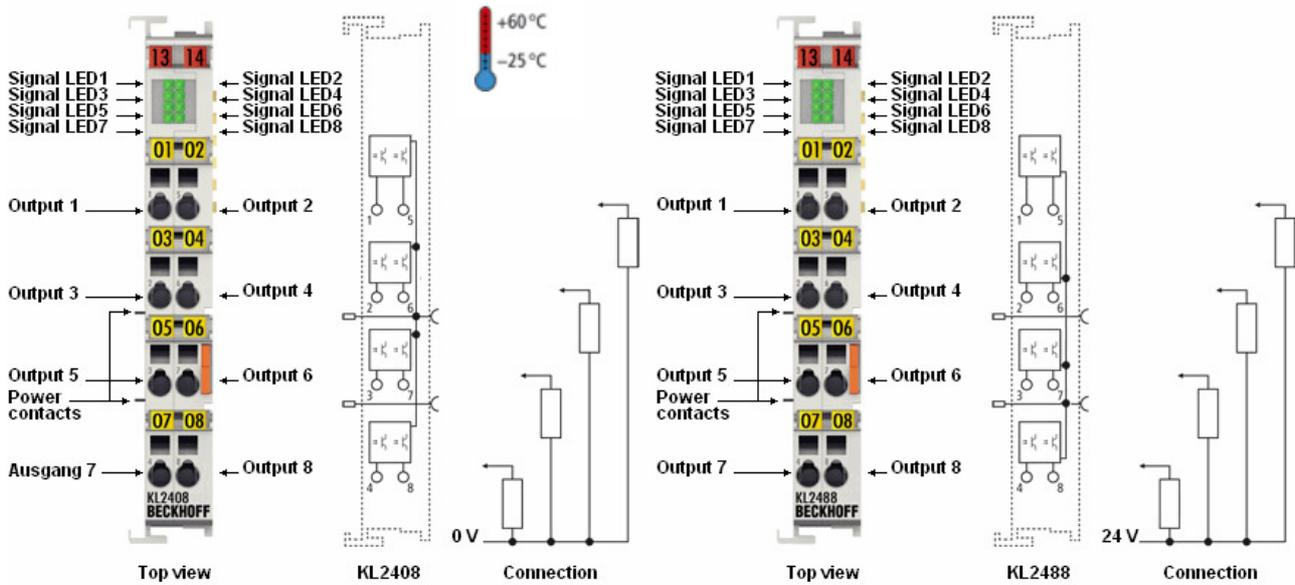
**Eight-channel, digital output terminal, 24 V<sub>DC</sub>**
