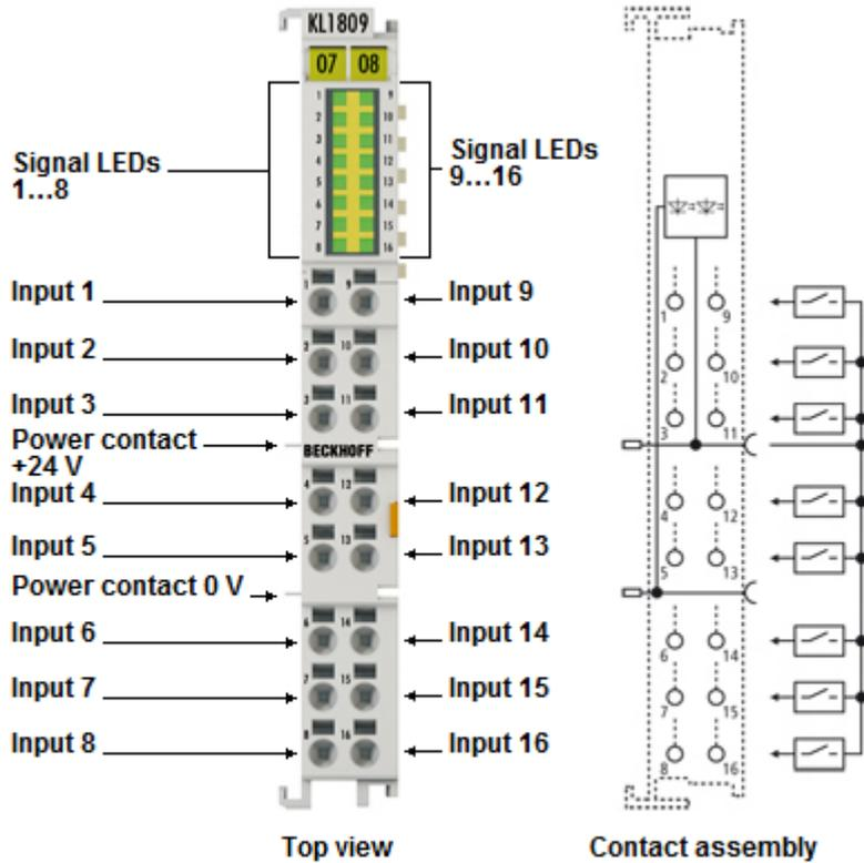
**KL1809, KL1819 | HD Bus Terminals, 16-channel digital input 24 V DC**
