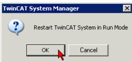
Fig. 186: Restarting TwinCAT in RUN mode
