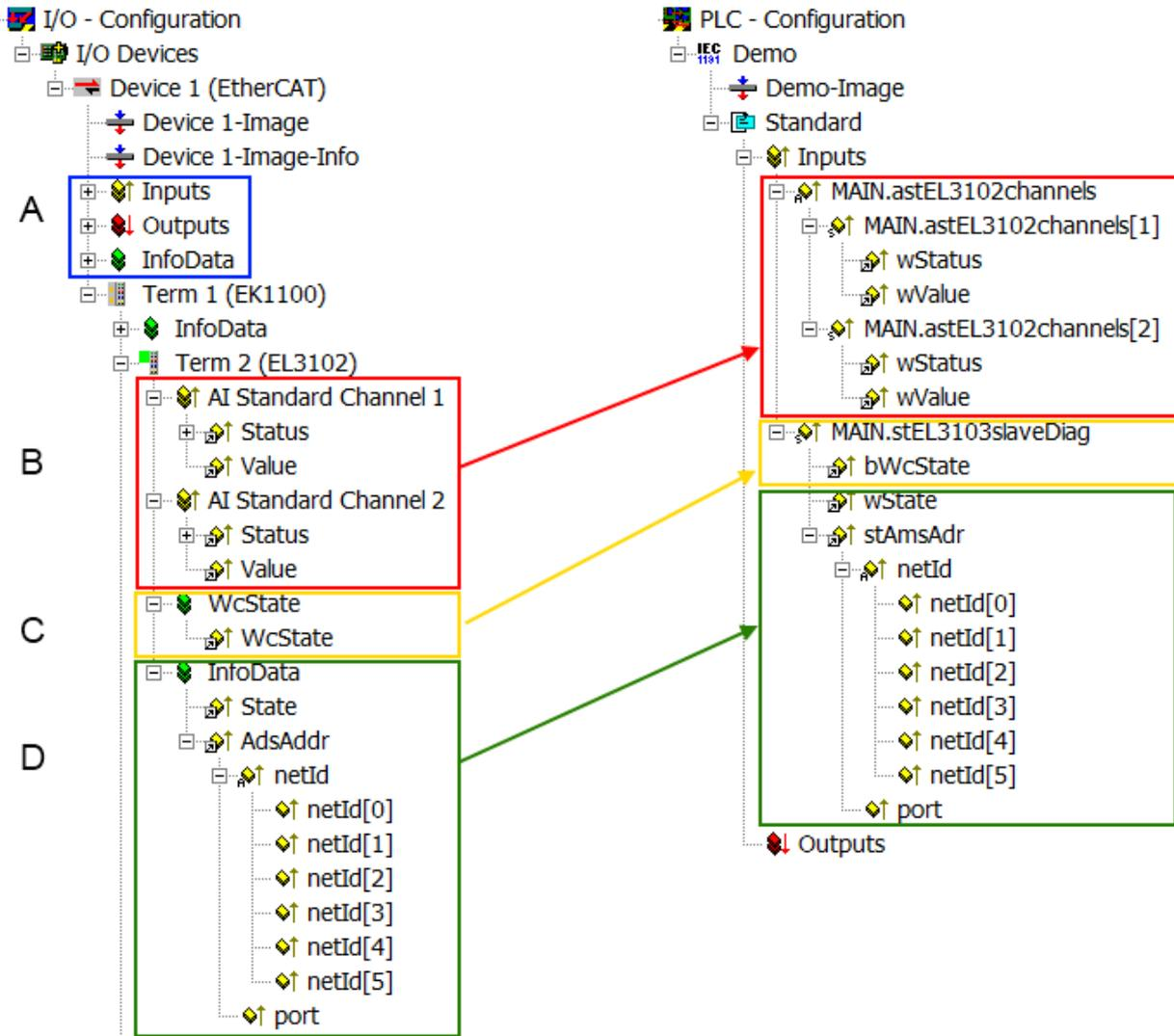
Fig. 95: Basic EtherCAT Slave Diagnosis in the PLC
