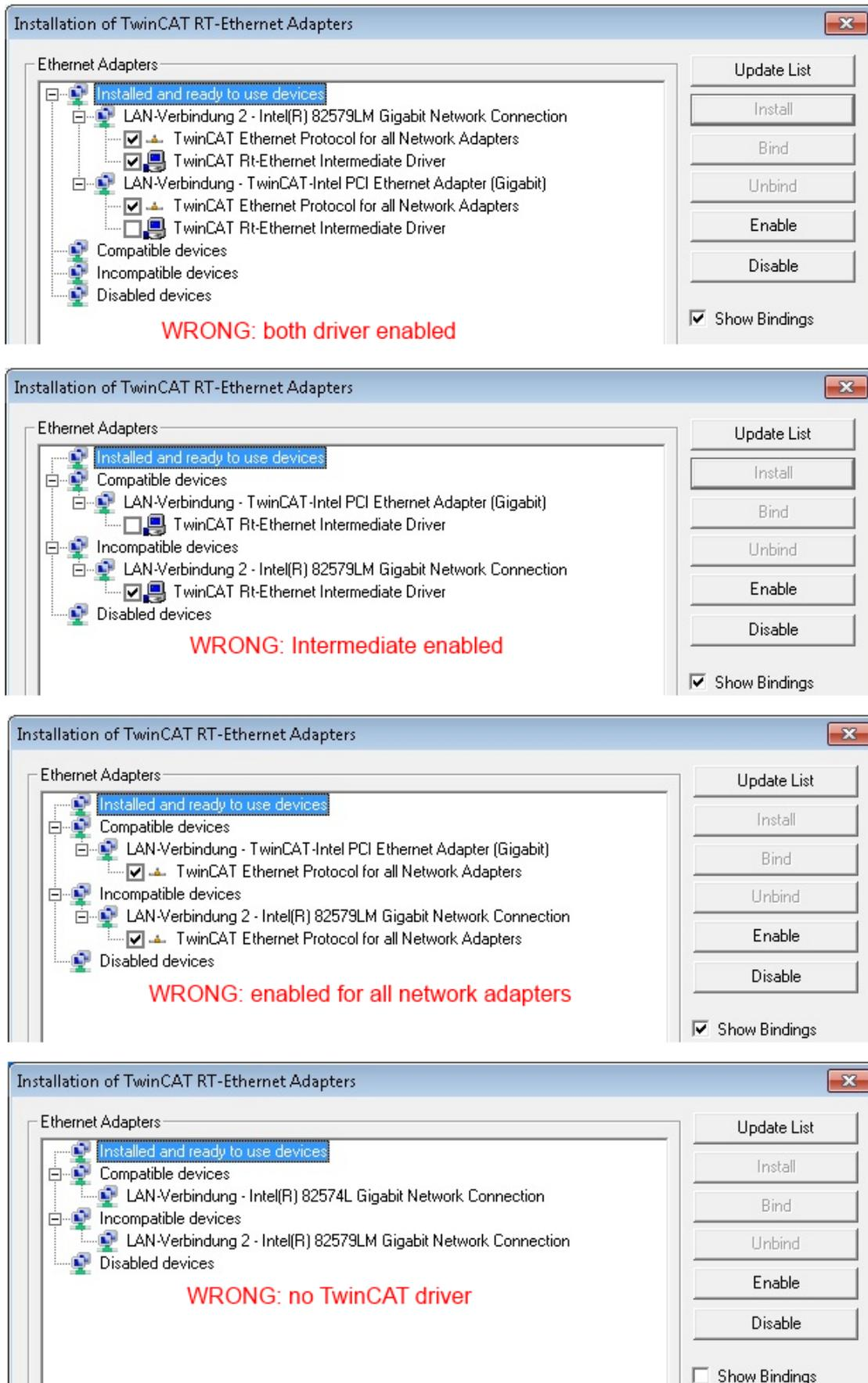
Fig. 50: Incorrect driver settings for the Ethernet port
