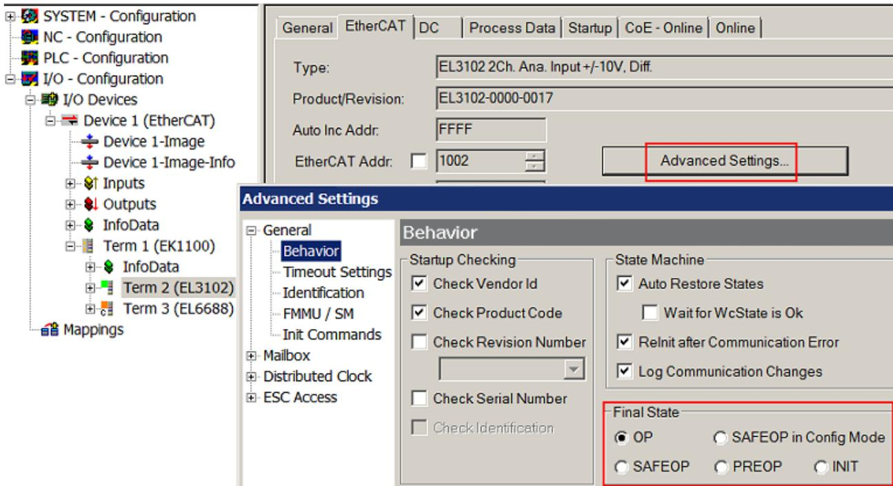
Fig. 99: Default target state in the Slave
