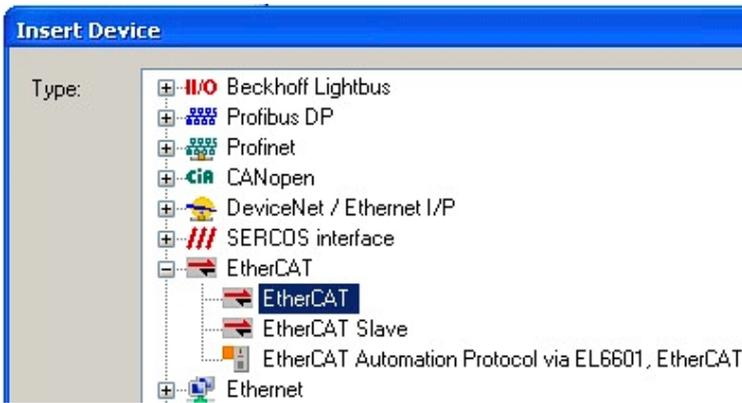
Fig. 59: Selecting the EtherCAT connection (TwinCAT 2.11, TwinCAT 3)
