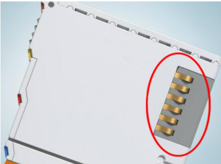
Fig. 31: Spring contacts of the Beckhoff I/O components
