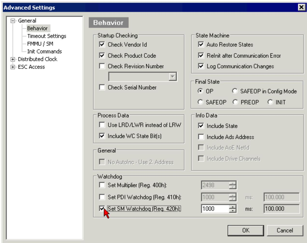
Fig. 29: eEtherCAT tab -> Advanced Settings -> Behavior -> Watchdog
