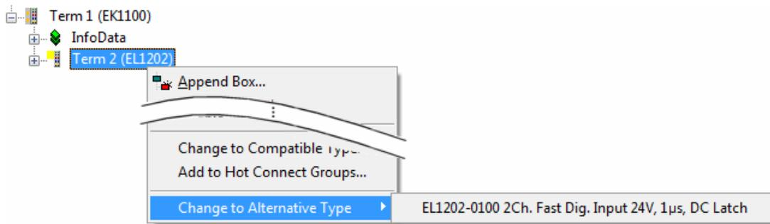
Fig. 88: TwinCAT 2 Dialog Change to Alternative Type
