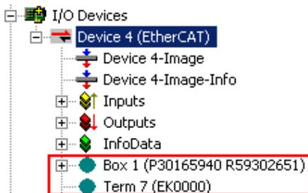
Fig. 82: Faulty identification
