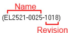
Fig. 52: Identifier structure
