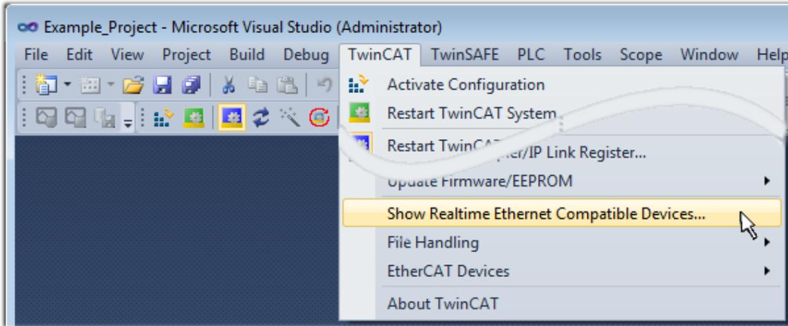
Fig. 44: Call up under VS Shell (TwinCAT 3)
