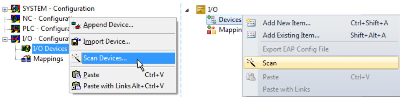
Fig. 69: Scan Devices (left: TwinCAT 2; right: TwinCAT 3)
