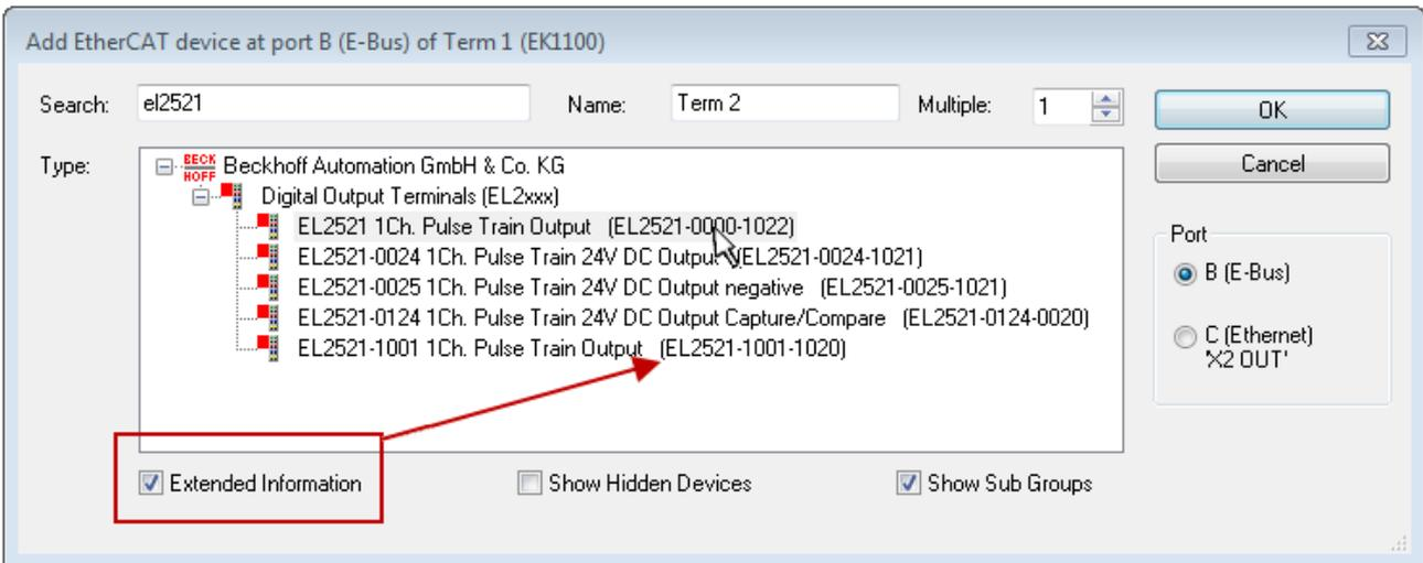
Fig. 64: Display of device revision
