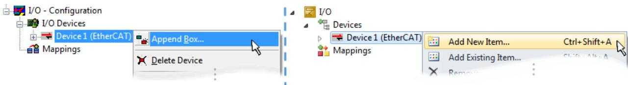
Fig. 62: Appending EtherCAT devices (left: TwinCAT 2; right: TwinCAT 3)
