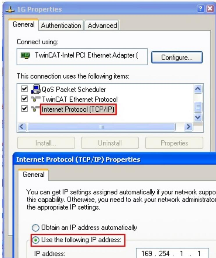
Fig. 51: TCP/IP setting for the Ethernet port
