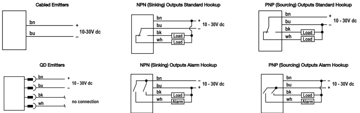
**Note:** Cabled hookups are shown. QD hookups are functionally identical.
